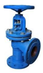
The body design of an angle pattern globe valve is characterized by its departure from the primary regular pattern globe valve. In this design, the opening and closing components consist of plug-shaped valve discs with a flat or conical sealing surface. The disc travels linearly along the fluid's centerline during the valve's operation. What sets angle globe valves apart is that their ends are positioned at a 90-degree angle, and fluid flow is achieved through a single 90-degree rotation.
